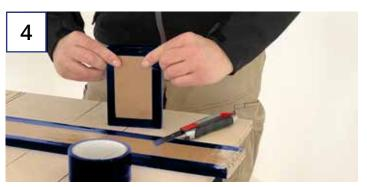
**FOLD OVER THE CORNERS** Fold the overlap at the corners downward and press the lateral overlap against the board surface.
